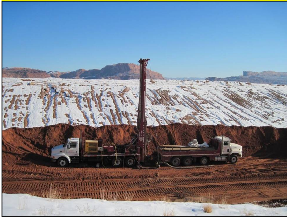
Photo 1. The DR-12 Air Rotary Drill Rig at Location 0453
