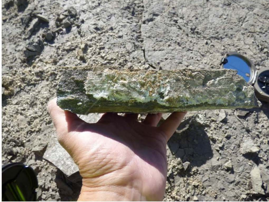
Photo 3: Precipitate on a bedding plane of the weathered Mancos shale.
