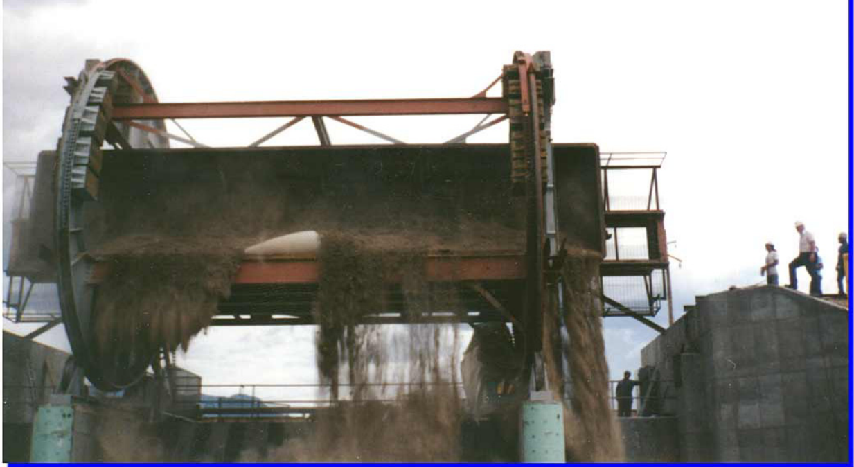
Figure 2–23. Operational Rotary Dump Facility
