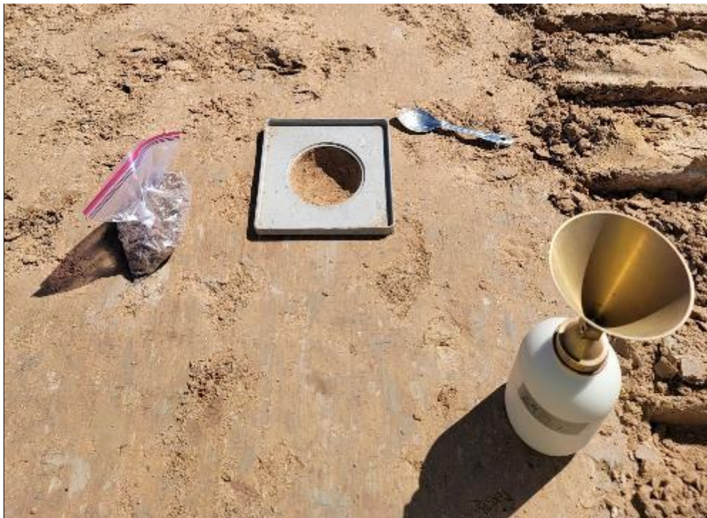
Photo 48. Preparing for Sand Cone Testing May 2021
