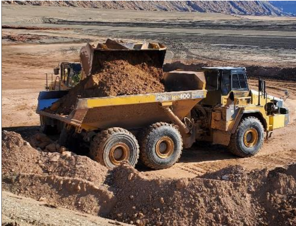
Photo 43. Loader Loading Material in Haul Truck April 2021
