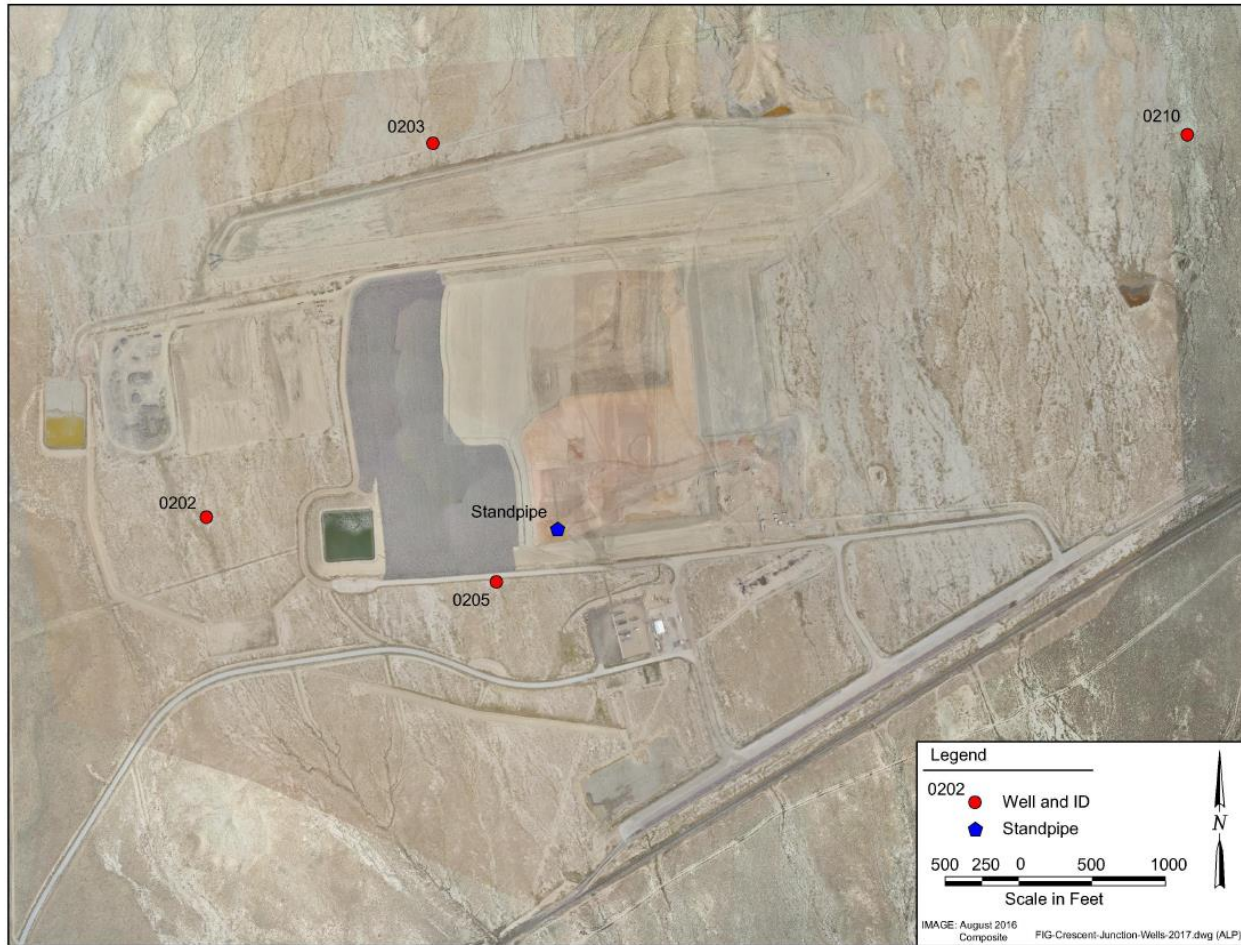
Figure 6. Locations of Monitoring Wells and Standpipe
