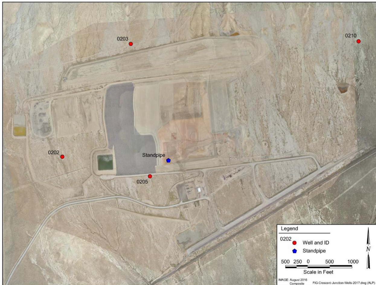
Figure 6. Locations of Monitoring Wells and Standpipe
