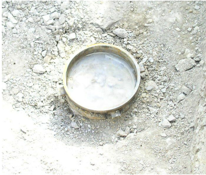
Figure 8. Frozen Hydration Water in the Non-Leaking AEP Test Performed in TP 0152
