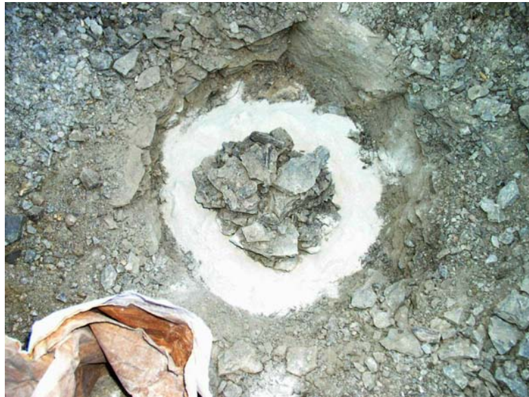
Figure 4. Sodium Bentonite in Bottom of Circular Channel Excavated into Weathered Mancos Shale
