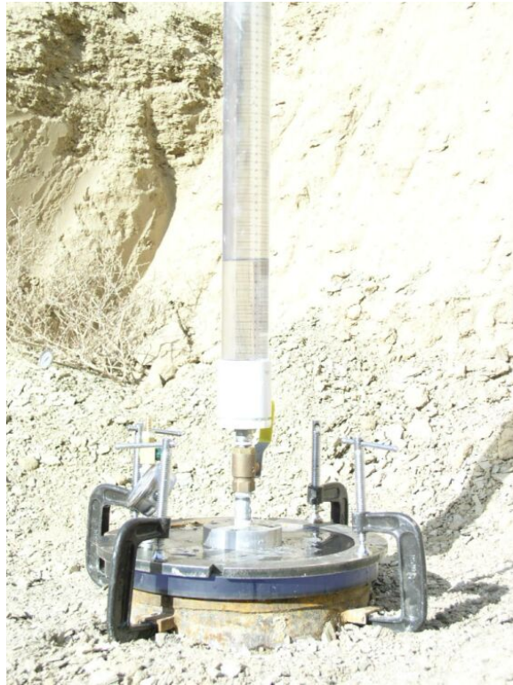
Figure 7. AEP Installed in wthrd K_m – TP 0154
