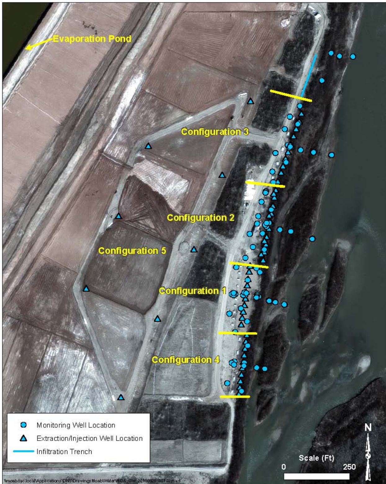
Figure 6. Locations of Select Monitoring and Extraction/injection Wells at the Moab Site
