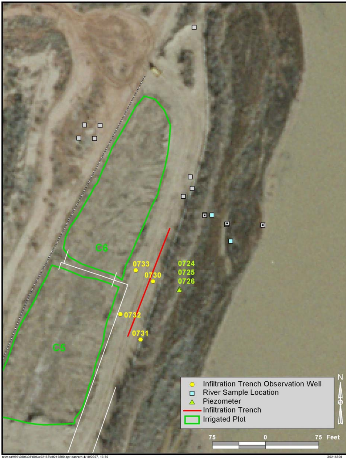
Figure E-1. Map View of Infiltration Trench and Sampling Locations
