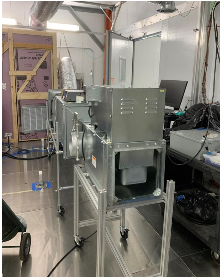
Code tester to measure air flow rate
