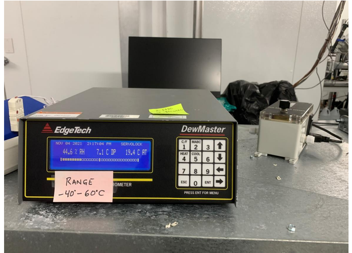
Chilled mirror humidity sensor to measure supply air dew point
