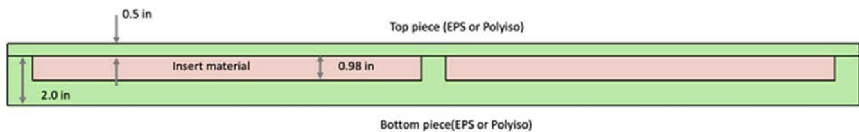
Figure 11: The cross section of the composite core insulation defined above shows a vacuum insulation panel with a thickness of 0.98 in. encapsulated in plastic rigid foam, expanded polystyrene or polyisocyanurate.
