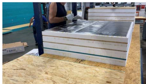
Figure 37: Visual and physical inspection should be done before the embedding into foam
