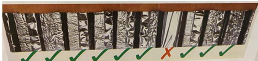
Figure 36: Visual inspection is key to identifying compromised or damaged VIPs
