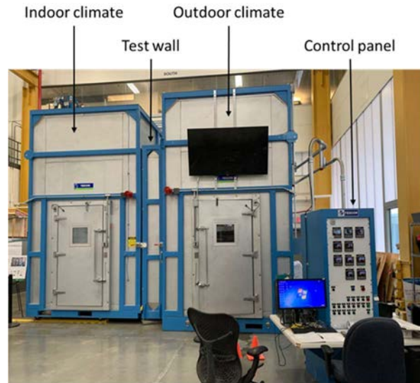
Figure 25: Heat, Air, and Moisture (HAM) chamber at ORNL. The chamber is comprised of two environmental compartments separated by a test frame that accommodates the wall assembly. The temperature and relative humidity can be controlled in both compartments.
