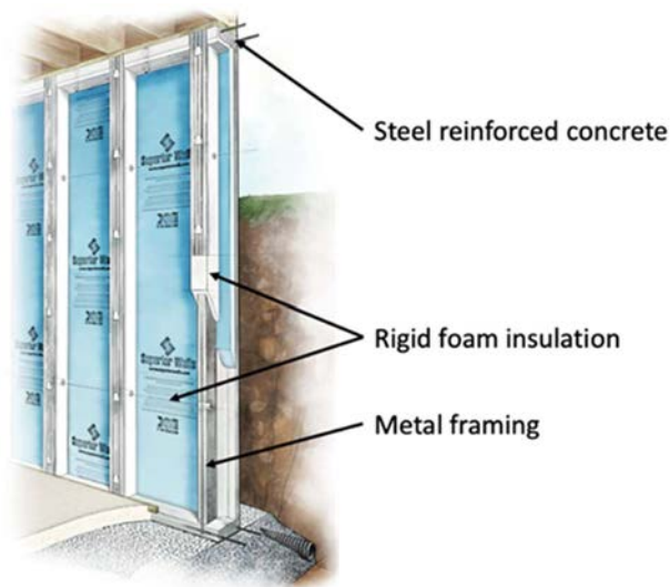
Figure 3: Precast Insulated Concrete Panel (Source: Superior Walls, https://www.superiorwalls.com/superior-walls-products/ )
