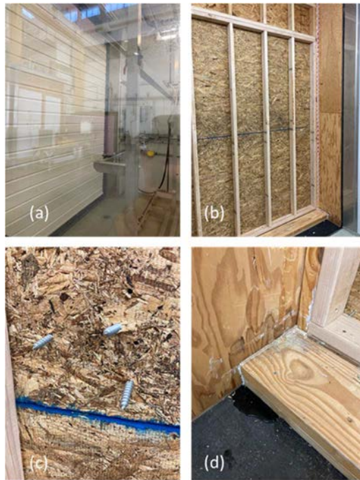
Figure 28: Results from water penetration test. (a) rain load being applied to the exterior cladding of the wall assembly. (b) is the interior of the wall assembly, no water penetration observed. (c) air leakage detected at fasteners. (d) water passing underneath the frame of the test panel. The water was not caused by passage of water behind the retrofit panels.
