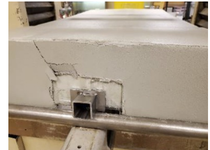
6A FIT Flexural Test Failure Mode Detail
