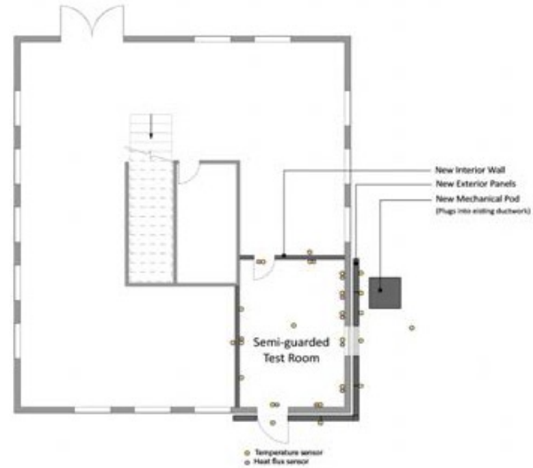
Sensor layout for interior zone of south-east test room for benchmark testing and measurements of full-scale installation
