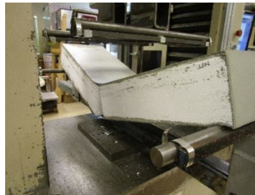
Top: 4A, 4B, 6A, 6B FIC Four-Point Loading Flexural Test Setup with 2" x 8" Wood Compression Plates.
