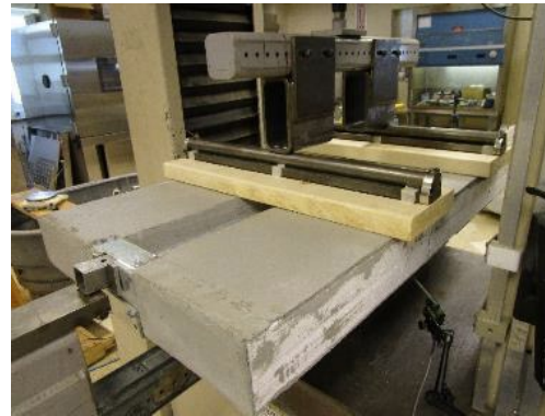
6A FIT Flexural Test Failure Mode Detail
