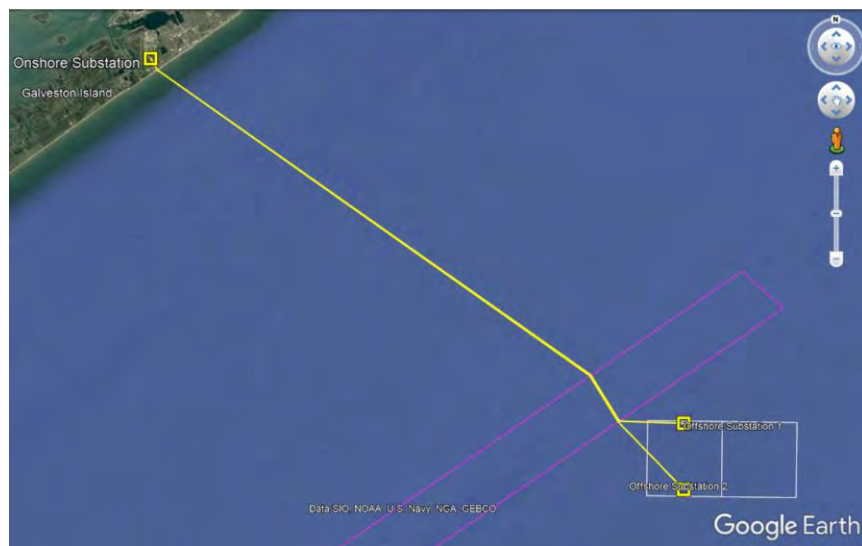
Figure 7. The export cable routes from the offshore substations to the point of interconnection.
