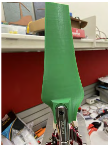
Figure 4: 3D printed blade model connected to pitch control
