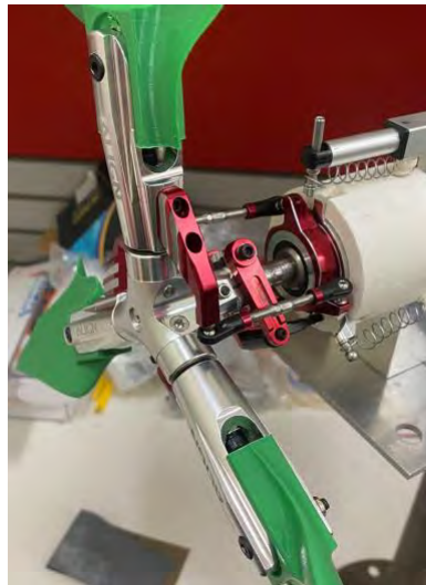
Figure 7: RC helicopter rotor repurposed for turbine pitch control.
