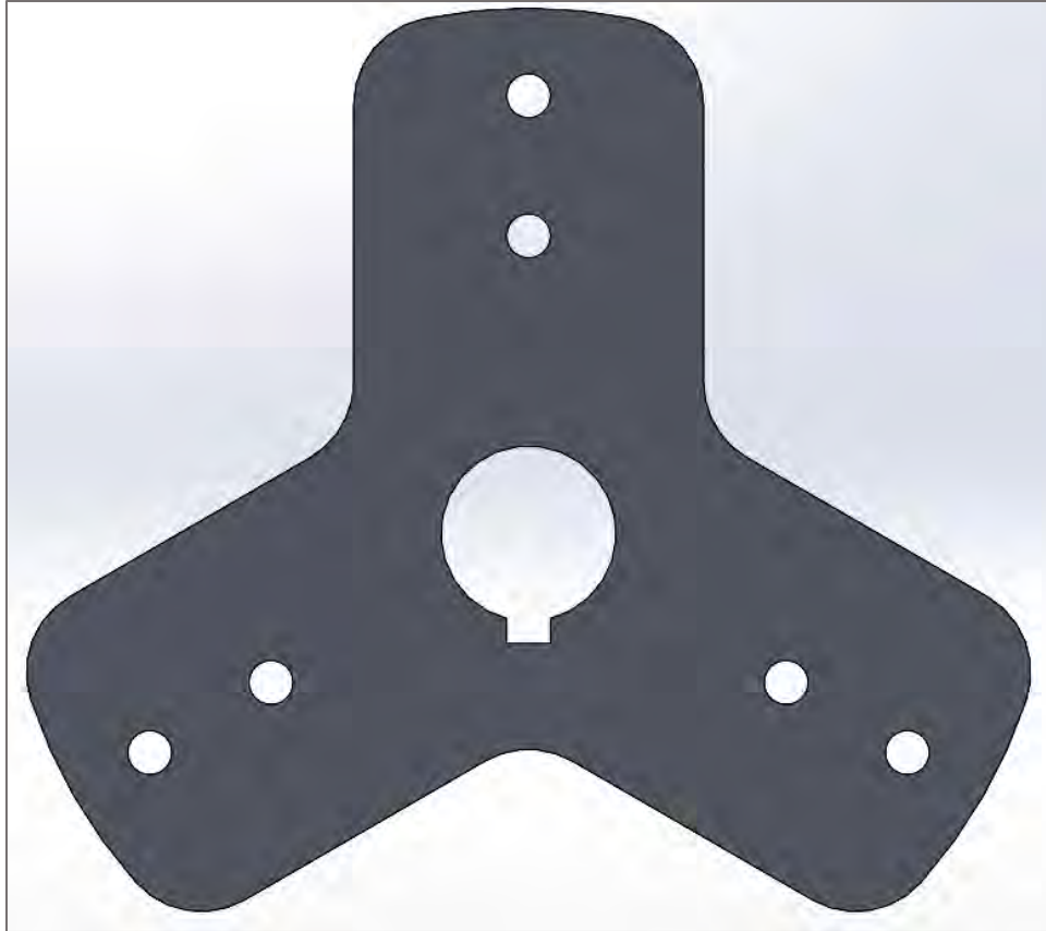
Fig. 4 Hub design with interfacing holes and keyway
