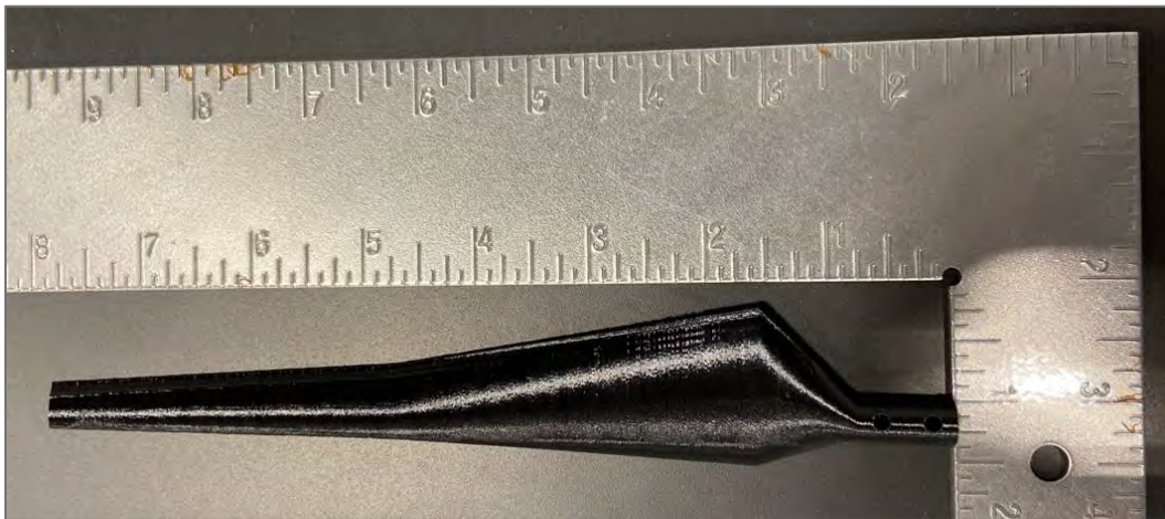
Fig. 3 Close-up image of a 3D-printed turbine blade
