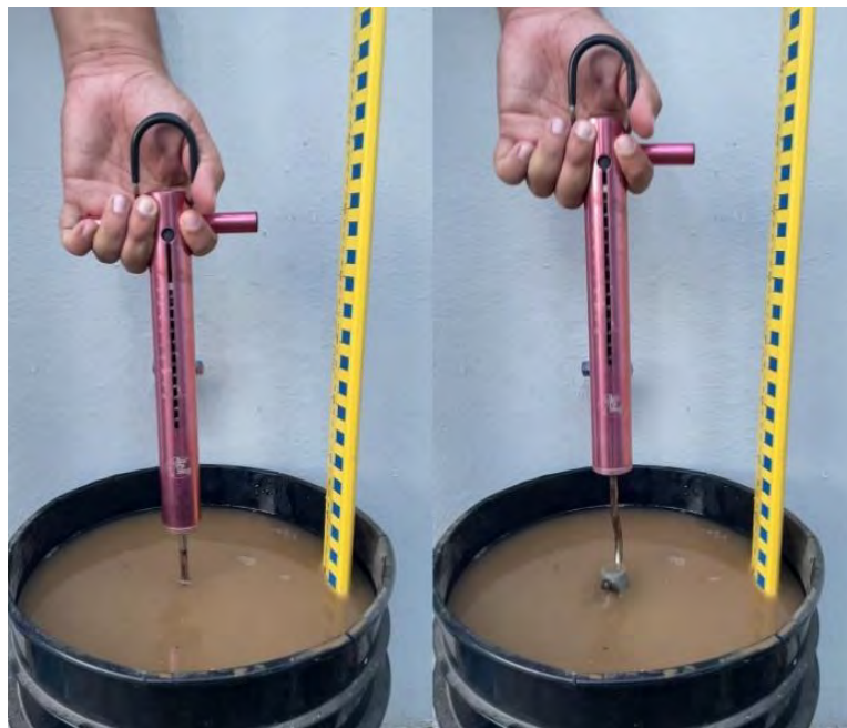
Figure 3. Single pile at maximum resistance and after breaking loose
