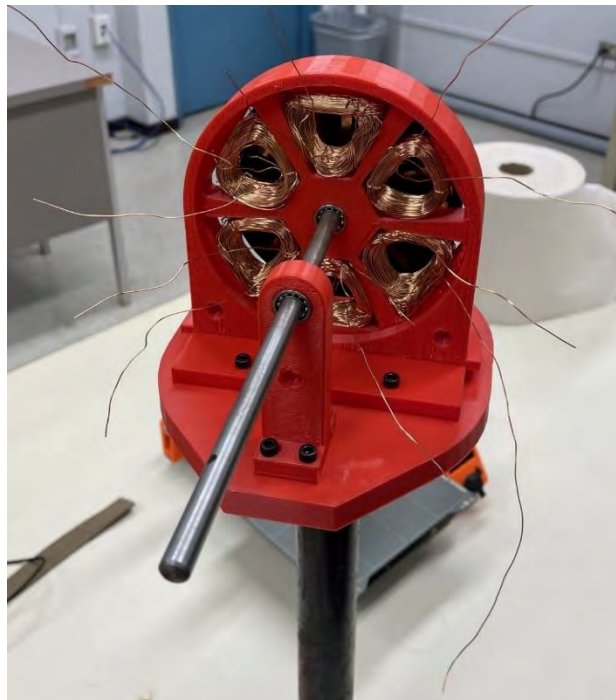
Figure 20. Generator Stator Assembly
