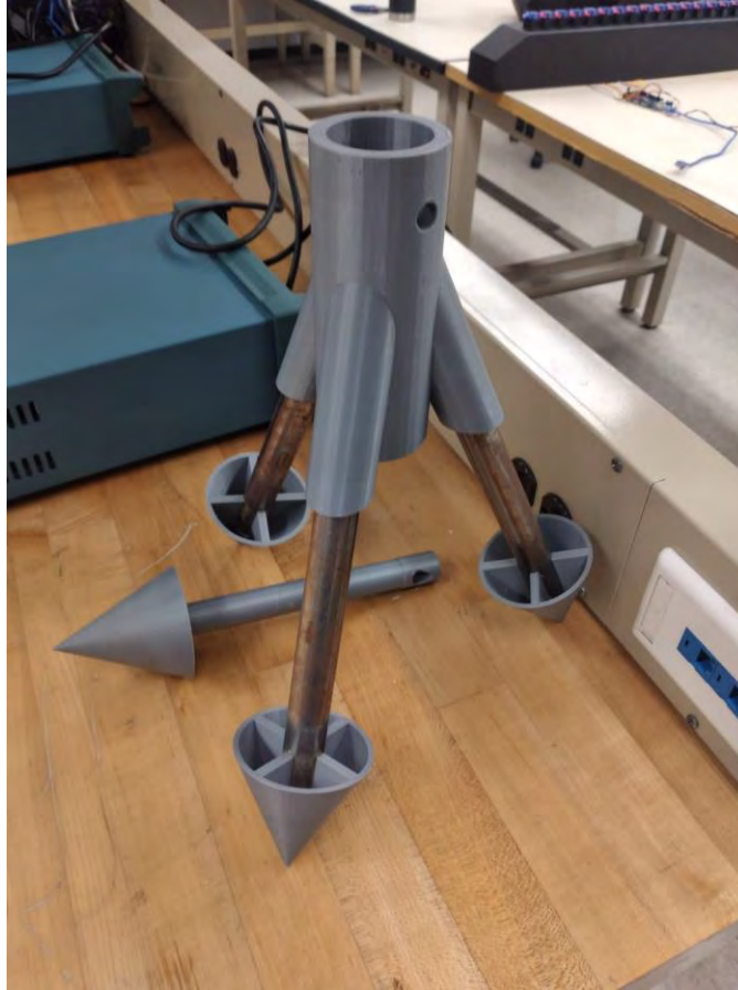
Figure 2. Foundation Tripod Assembly and Single Pile Below
