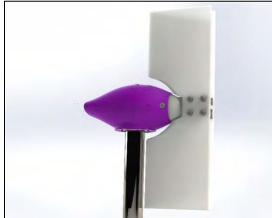
Figure 5: Nacelle SolidWorks Render w/ Tail Fin
