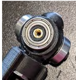
Figure 7: Heat Set Insert Installed on Nosecone
