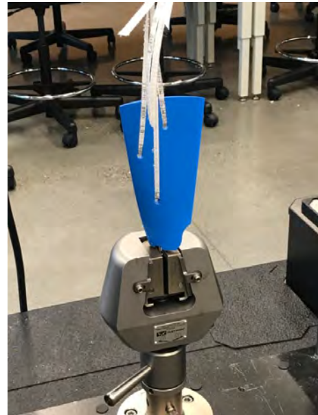
Figure 22: Wide Blade in a pull-test.
