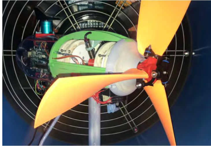
Figure 8: Angle view of EWET's final prototype wind turbine for the 2022 CWC competition.
