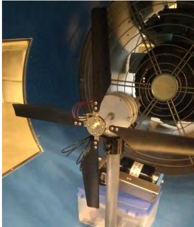
Figure 27: Wind tunnel testing of the single stack to determine KV rating.
