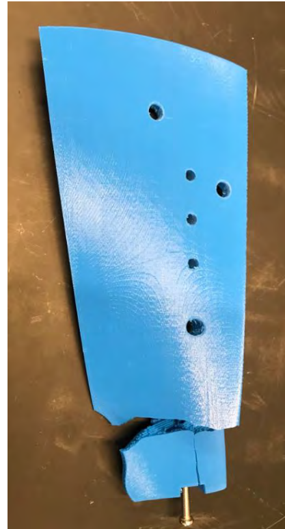
Figure 24: Post Test Remains after 2600 N of force.
