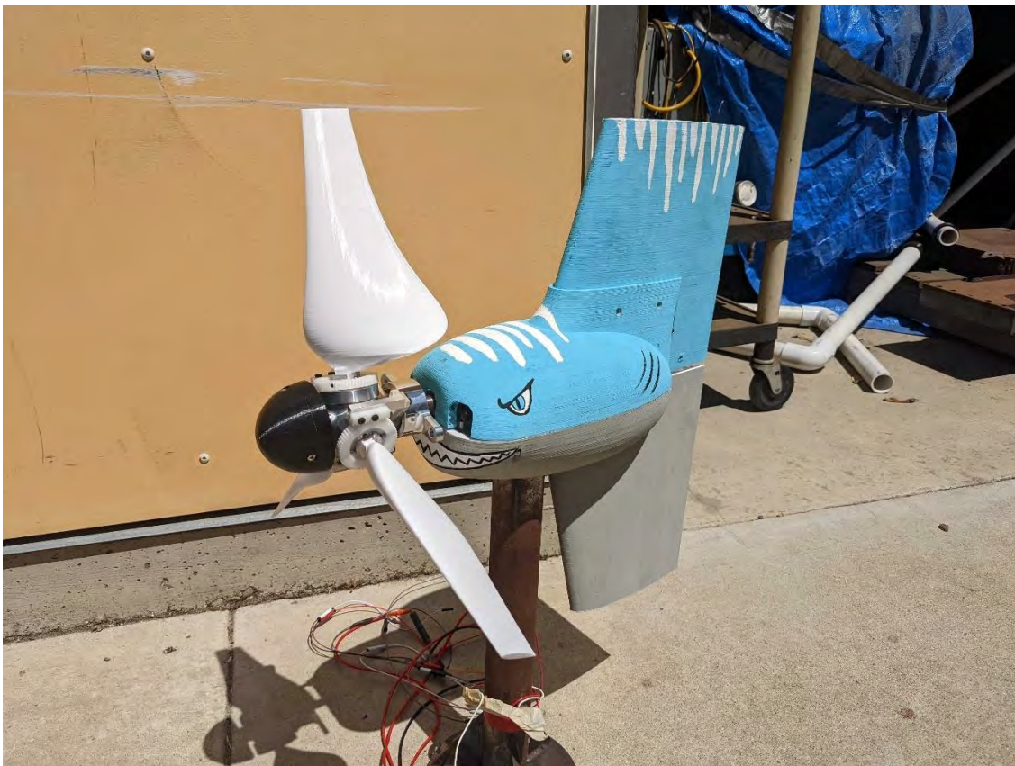
Figure 1: The completed turbine, YAWS, on the dry land testing tower.
