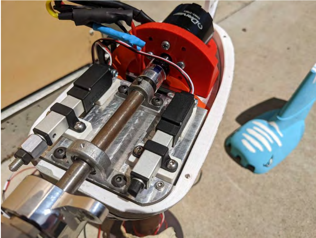
Figure 8: The drivetrain assembly and linear actuators for the pitching mechanism, most of which were maintained between years.
