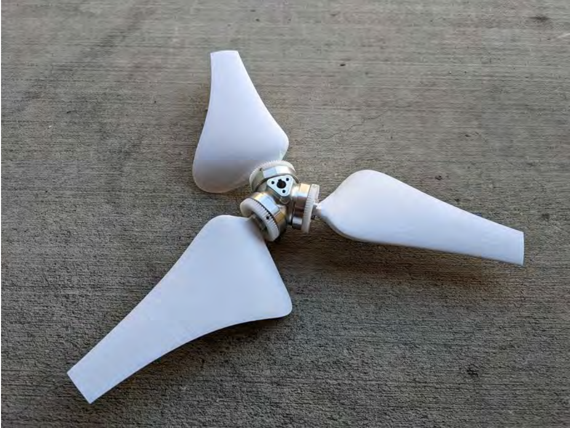
Figure 7: The final blade design situated into the pinions of the pitching mechanism. This unit is mounted onto the shaft and a nose cone is placed upwind for best airflow.
