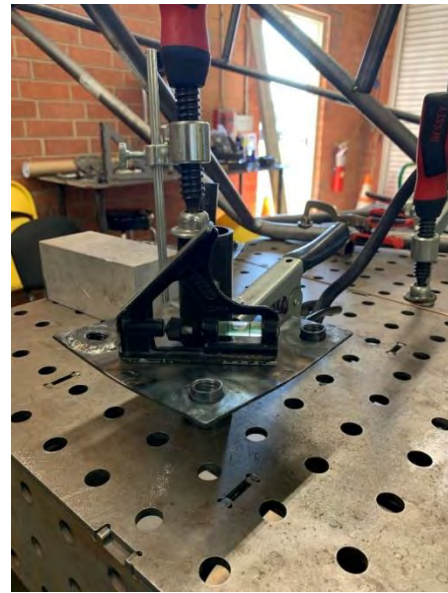
Figure 4-2 Leveling the Scribe - TIG Welding
