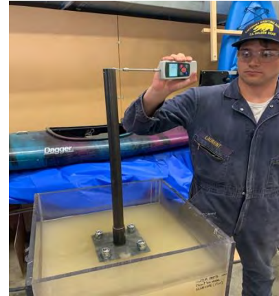
Figure 4-8 Foundation Assembly Testing
