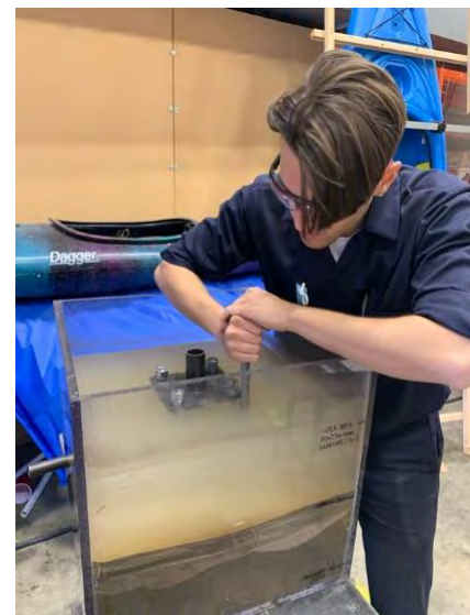
Figure 4-10 Packing the Sand
