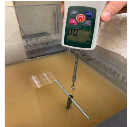
Figure 4-4 Anchor Tension Testing
