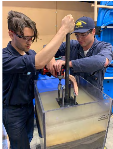
Figure 4-9 Impact Driving the Anchors
