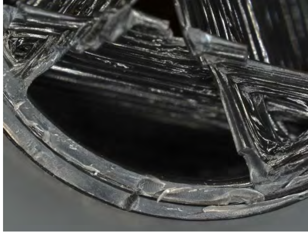
Figure 8 - Beach marks along failure surface of PLA blades
