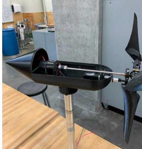
Figure 10 - View of the interior of the 3D printed nacelle.
