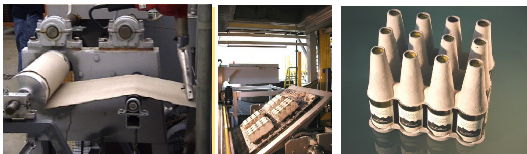
Figure 10. Processed paper and packaging products from MSW-derived fiber materials
