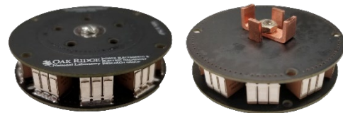
Figure 2. Assembled capacitor package: top view (left), bottom view (right).
