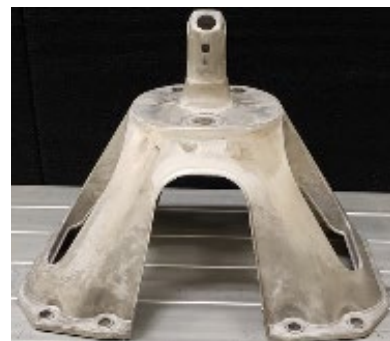
Figure 2. Image of spare tire carrier to be fabricated by Leggera Technologies using two scaled up, developmental alloys.
