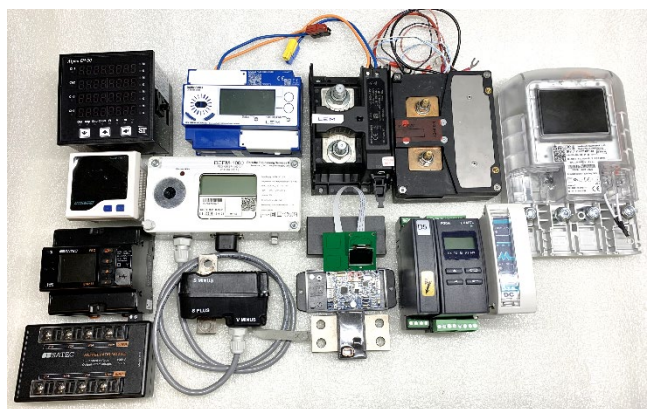
Figure 1. Tested 1000V/350A HB44-3.40 compliant DC meters.
