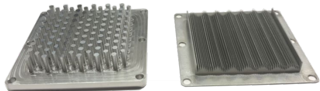
Figure 2. Prototype of the optimized heat sink design (right) in comparison to pin-fin heat sink (left).
