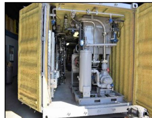
Containerized nitrogen equipment (8' x 40')
