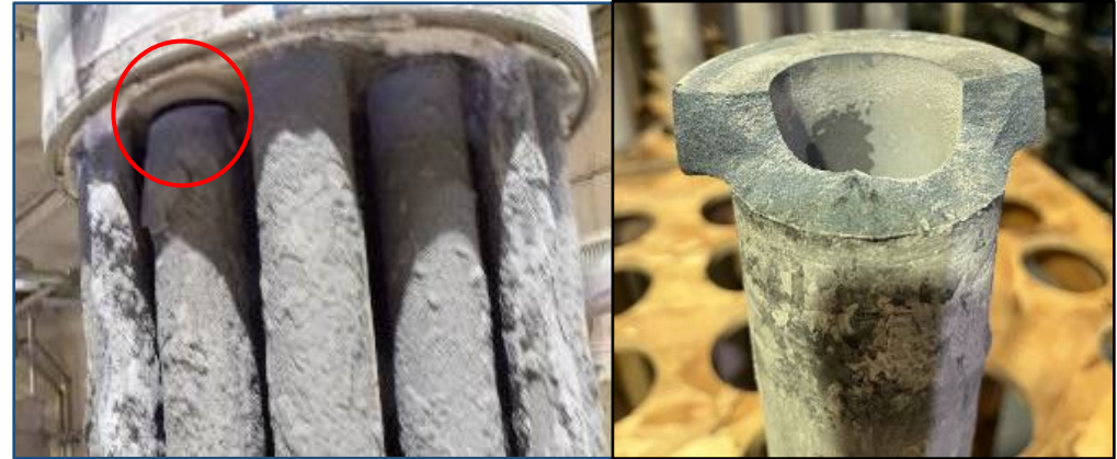
Two broken elements in bundle #16 Sent for failure analysis at Dominion Engineering
