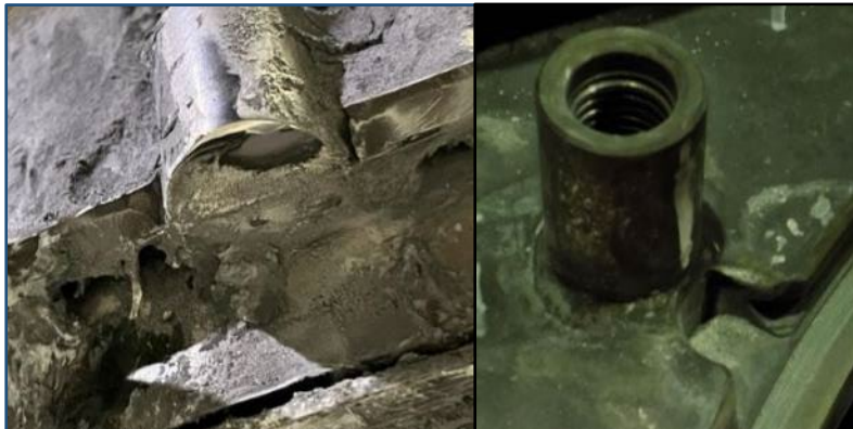
Potential interference between sub tubesheet and main tubesheet; debris inside tie down lugs
