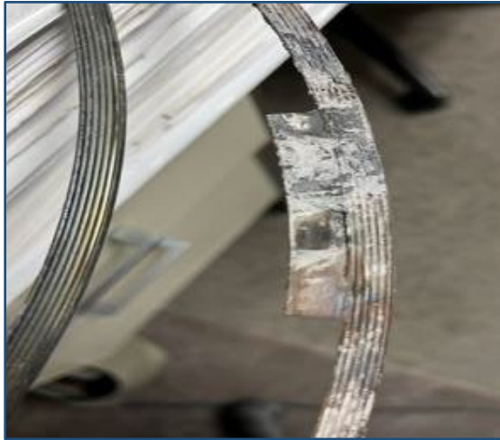
PGF bundle main gaskets intact but showed evidence of bypass
