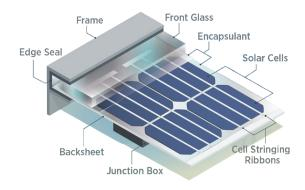
Figure 4. Components of a silicon module.
