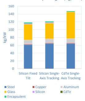
Figure 2. System-level materials breakdown by weight for fixed tilt and single-axis tracking configurations for a Si PV plant, and a single-axis tracking CdTe plant.
