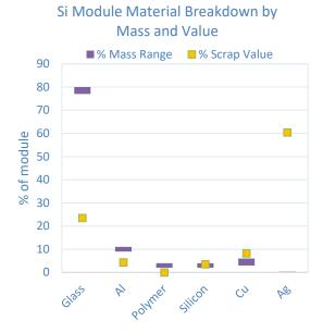
Figure 5. Material breakdown of a PV module by mass and by recoverable value.
