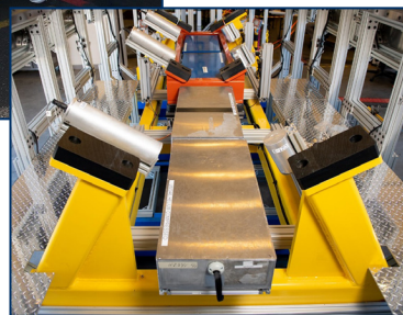
Inside the UCVS, the yellow metal framework and black pads cradle the UF 6 cylinders, much like a boat trailer, while the neutron detectors (rectangular metal running the length of the cradle in the middle of the photo and along the sides) and gamma detectors (silver “cans” positioned at angles the length of the cradle) scan the contents of the cylinder. Photo credit: Andrea Starr, PNNL
