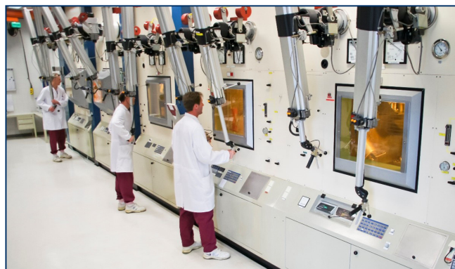
Operators processing Mo-99 in Curium's LEU hot cell which fully replaced HEU-based production in the Netherlands in 2018.
