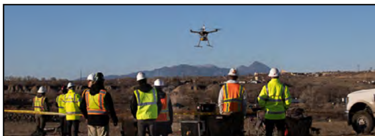
A drone takes flight to begin the baseline aerial survey at Shiprock, New Mexico.
