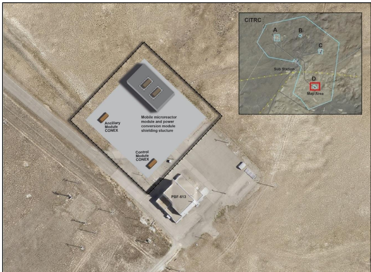
Figure 2.3-9. Mobile Microreactor Located at CITRC Test Pad D
