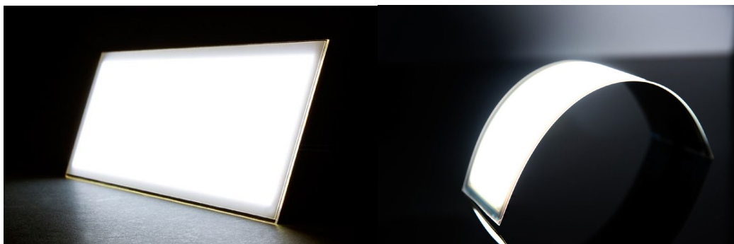
Figure 2.13 A rigid and flexible OLED light, respectively. The flexible light can be bent with a radius of curvature of 10 cm or higher. [13] [14]
