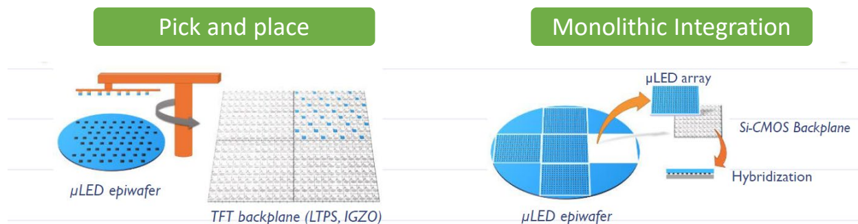
Figure 5.13 Schematic illustration of the micro-LED transfer onto a TFT backplane and the monolithic integration of a micro-LED array on a CMOS backplane. [194]
