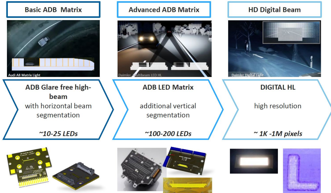
Figure 3.48 Comparison of different generations of adaptive driving beam (ADB) headlights showing the improving resolution with increasing pixel density. [83]
