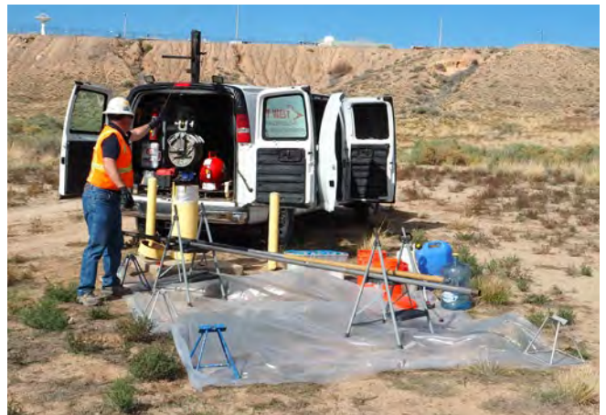
Geophysical logging at groundwater monitoring well TA2-W-19 on the Tijeras Arroyo floodplain.
