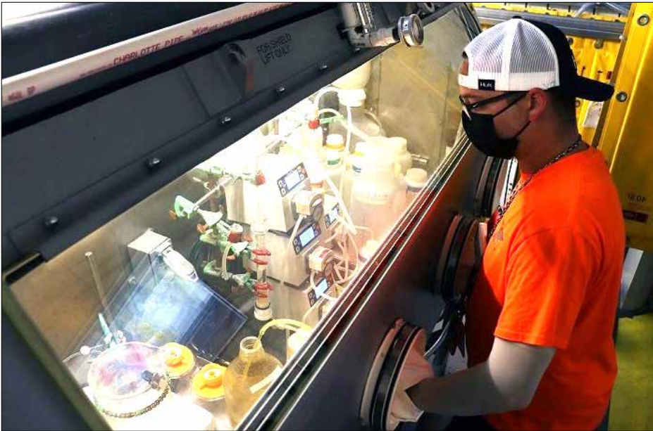
An Isotek employee processes low-dose uranium-233 material in a glovebox at Oak Ridge National Laboratory.
