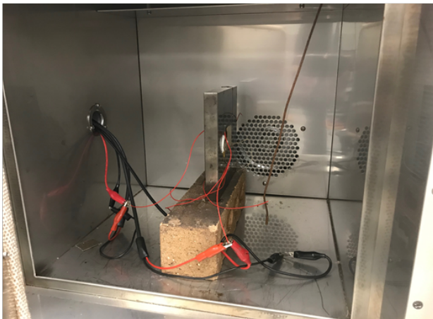
Fig.2 . Through wall communication modulus in a oven.
