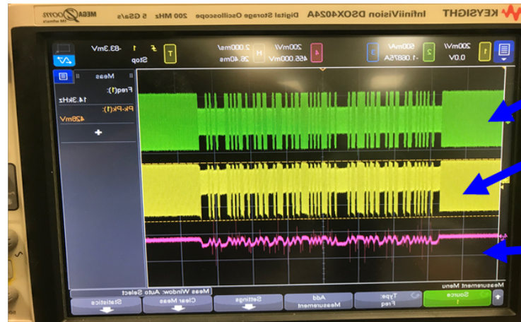
Fig. 3 . Through wall communication result (carrier wave frequency=100 kHz)
