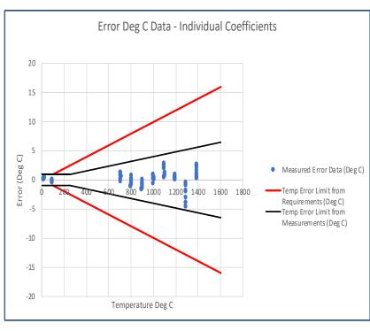
Error Requirement: 1% (16 Deg C at 1600 Deg C), Error Measured: < 0.4% (6.4 Deg C at 1600 Deg C
