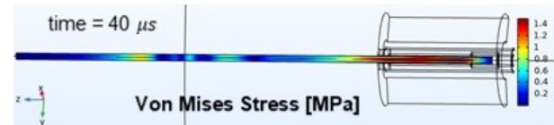
FEA model of 1.6 mm waveguide UT
