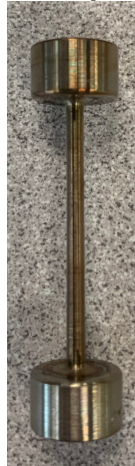
Creep Test Rig post autoclave testing
