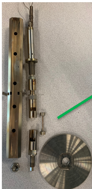
Creep Test Rig post autoclave testing
