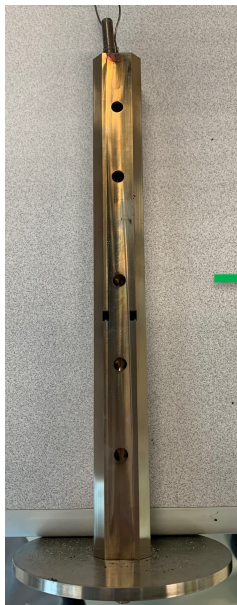
Creep Test Rig post autoclave testing
