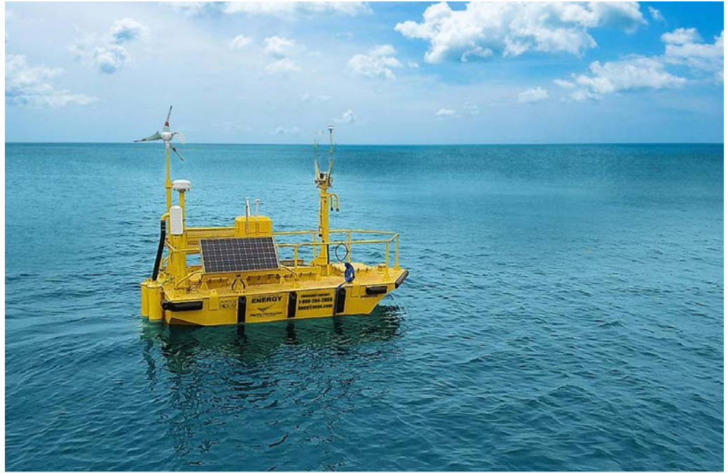
U.S. Department of Energy lidar buoy deployed off Morro Bay, California. Photo from AXYS Technologies and Pacific Northwest National Laboratory (PNNL)
