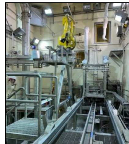
Canister decon robot undergoing testing inside the Can Fill Cell
