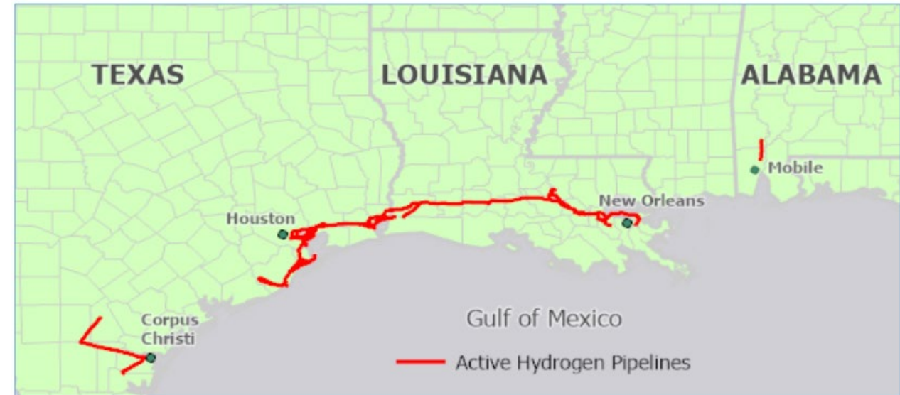
Existing Gulf Coast Hydrogen Pipelines
