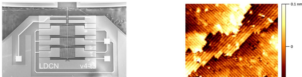
Figure 26. A silicon-on-insulator (SOI)-MEMS on-chip STM (left) and image of an H-passivated Si surface acquired with this device (right).
