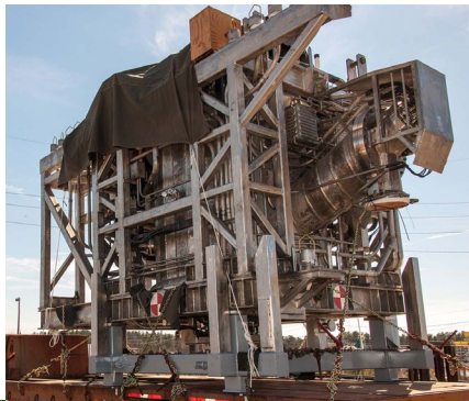
Left: Spare Melter for Waste Vitrification at DWPF.
