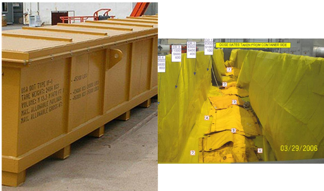
Figure 2-1. Exterior of B-36 Disposal Container and Actual Tank 28F Salt Sampling Drill String and Lead Blankets in B-36
