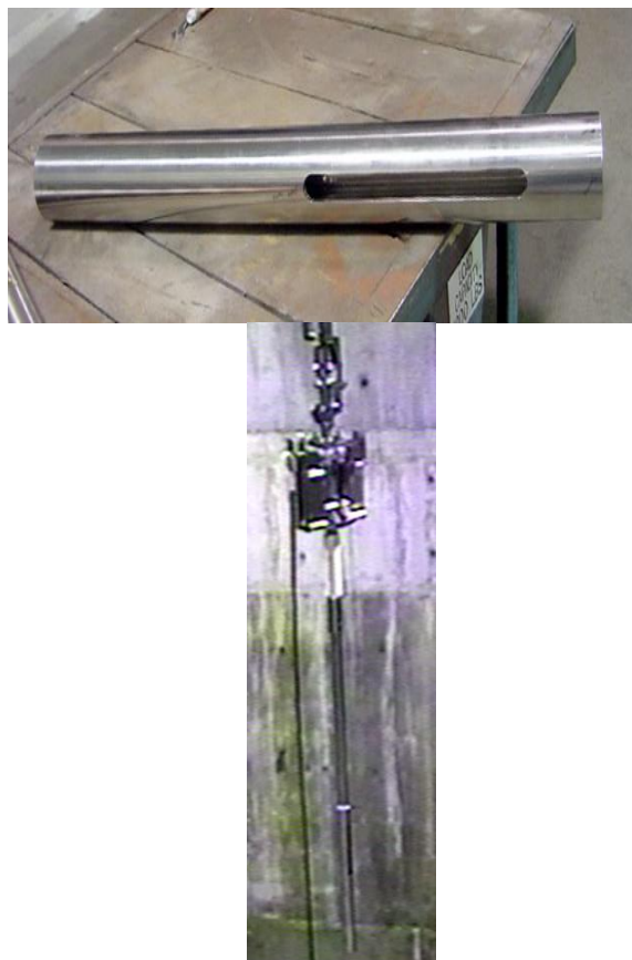
Figure 2-3. Close-up of Inconel Pipe (a) and Glass Pump (b)
