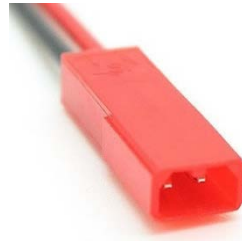
Figure 14. Team-provided connection to the manual shutdown interface
