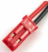
Figure 15. Competition-provided connector for manual shutdown interface
