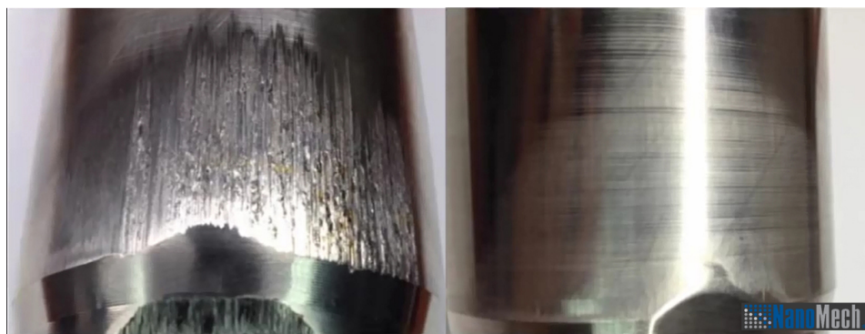
Component wear with (left) and without (right) the nanoengineered lubricant additive (Image courtesy of NanoMech)
