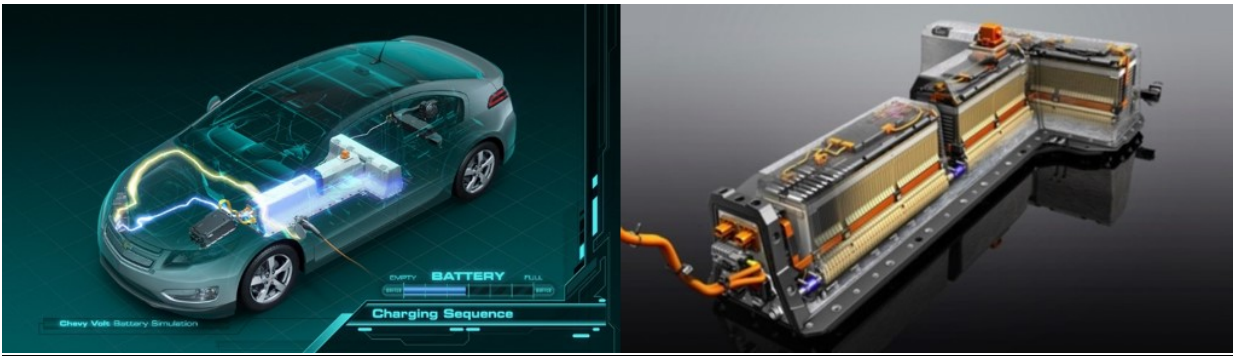
Large T-shaped battery charging in the Chevy Volt (Image courtesy of General Motors)
