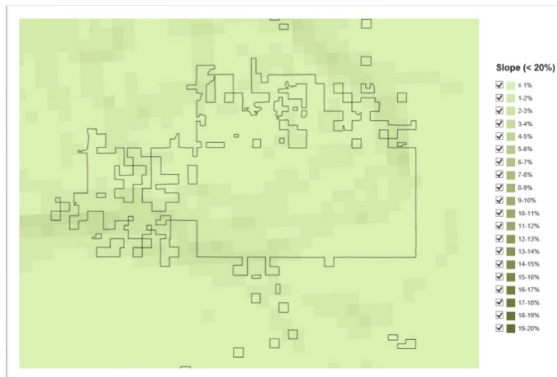
Figure 3-2. Maximum Percent Slope of Turtle Mountain Tribal Lands at 1 km Spatial Resolution (NREL Wind Prospector)
