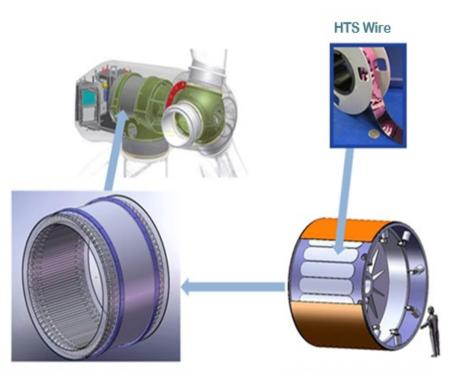
Copper Stator with Back Iron
