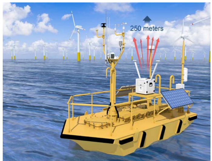
One of two offshore wind research buoys that are managed by PNNL, as depicted in an artist’s rendering. The buoys are equipped with instrumentation that can take wind speed measurements as high as 250 meters, the height of today’s wind turbines. Results will help wind power plant operators make decisions for states such as California on investments and locations. Image by Mike Perkins, PNNL
