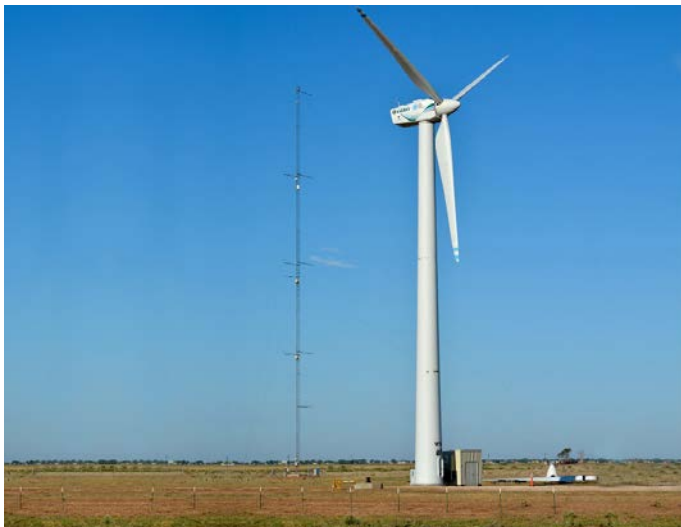
The National Rotor Testbed turbine is designed to help wind power plant operators understand how they can lower energy costs using wake control approaches. Photo by Chris Kelley, Sandia National Laboratories
