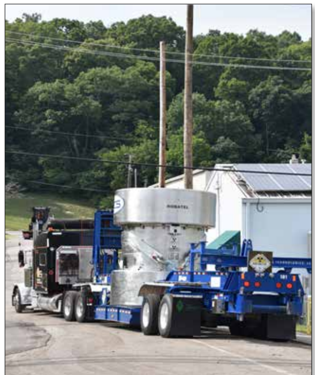
Next, they inserted the sealed liner into a second liner, (left) which was then loaded onto a specialty holding system (below) designed to ensure safe transportation for offsite disposal.
