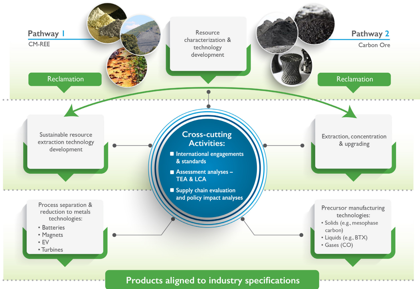
Figure 3. Coal-based Material Flow Chart for Co-production of CM and Carbon Products
