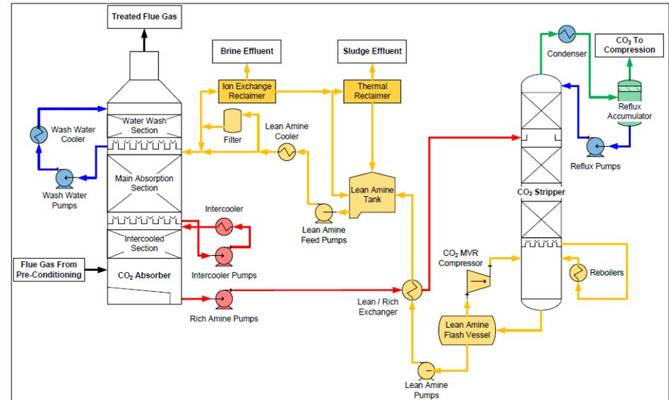
Process Flow Diagram of Shell's CO<sub>2</sub> Capture Process
