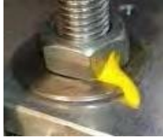
Figure 13. Marked nut and washer for torque audit
