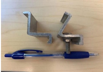
Figure 26. Bent module end clamp (right) compared to an unbent end clamp (left)
