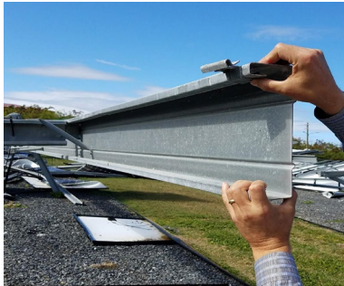
Figure 36. View showing clamp size compared to the structural element
