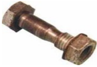
Figure 22. Bolt shaft worn out by joint movement
