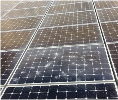
Figure 54. Module with broken glass top-sheet
