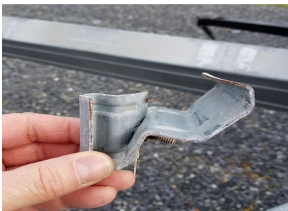
Figure 37. Damaged clamp used to hold structural elements together
